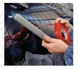
transfer. The carriers determinate part of double-sided adhesive performances such as conformability, thermic resistance, cohesive force of the tape, rigidity and other factors like the cut resistance, the kind of elongation, the handiness, etc.
